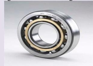
A leading bearing manufacturer states that the life of bearing oil is directly related to heat. Non contaminated oil cannot wear out and has a useful life of about thirty years at thirty degrees centigrade. They further state that the life of the bearing oil is cut in half for each ten degree centigrade rise in temperature of the oil.
