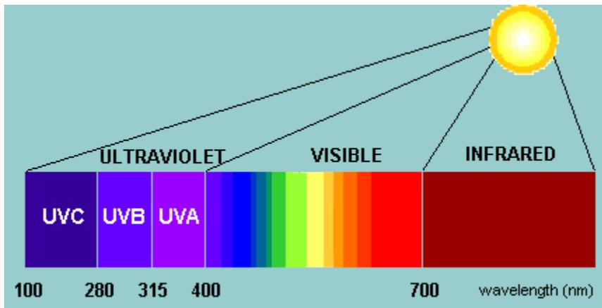
**Figure 2 Ultraviolet Range of the Electromagnetic Spectrum**
