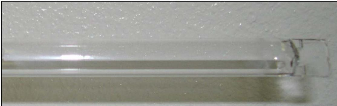
The lamps operate at between 60 – 80 degrees Celsius. A small fan is used to evacuate warm air from inside the quartz sleeve. This helps to ensure that the quartz sleeve is at the same temperature as the surrounding water reducing fouling and eliminating the potential for overheating in periods of low flow or if the water level drops. This can be seen in the diagrammatic representation of a drinking water system in Figure 6.
