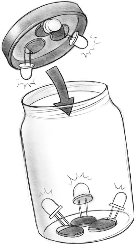
③ Use the tape to attach the LEDs to the inside of the jar. I put some on the lid and some on the bottom.
